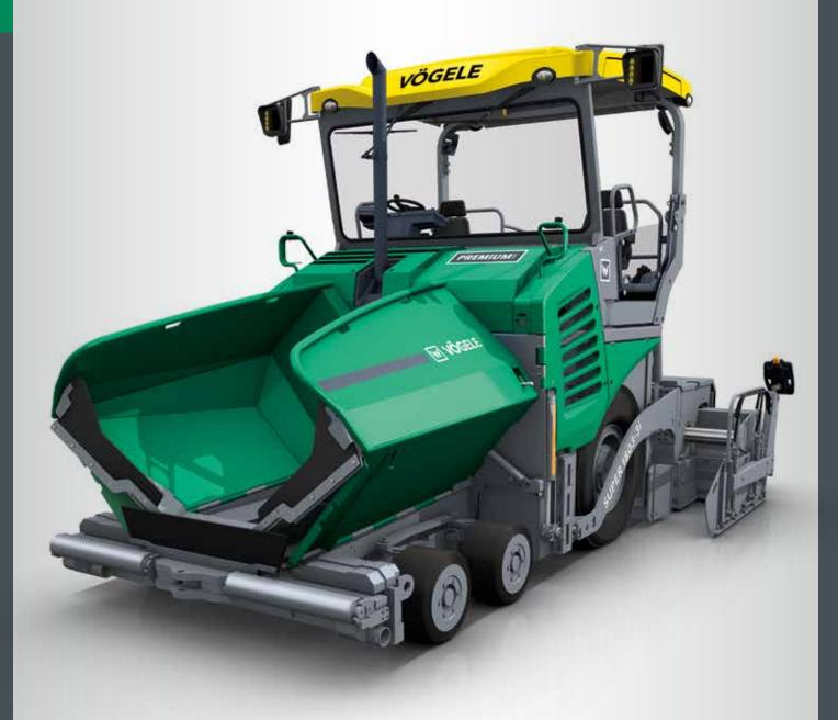
Maximum pave width 8 m Maximum laydown rate 700 tonnes/h Transport width 2.55 m
