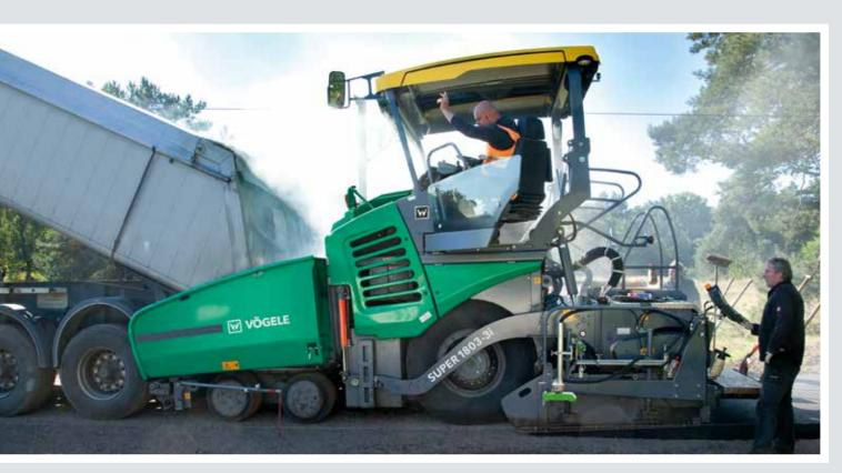
The power unit of the SUPER 1803-3i with its diesel particulate filter (DPF), diesel oxidation catalyst (DOC) and selective catalytic reduction (SCR) for exhaust gas after-treatment complies with the strict requirements of European exhaust emissions standard Stage V and US EPA standard Tier 4f.
