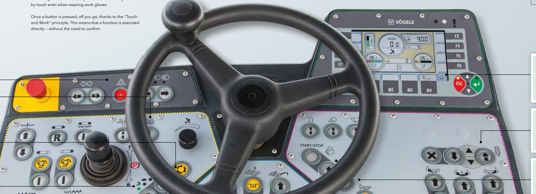
Module 1: Conveyors and augers, traction
