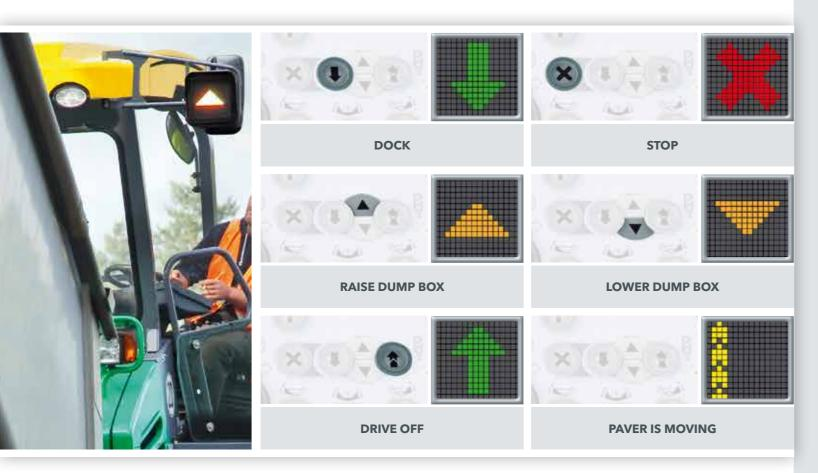
**The core element** of the PaveDock Assistant are the signal lights on the paver and the associated control elements on the paver operator's ErgoPlus 3 console.
