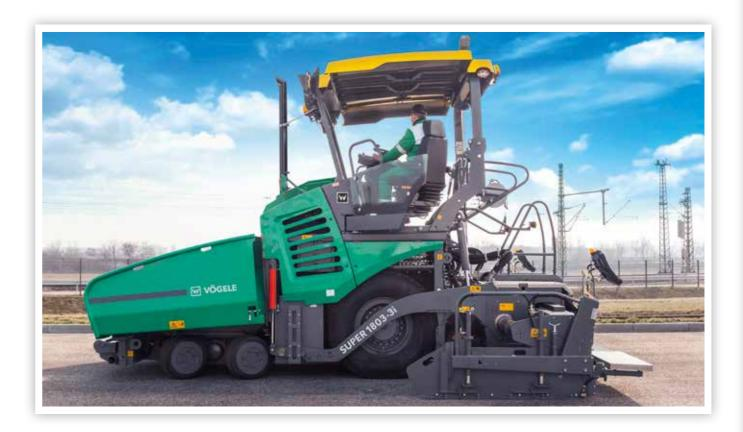
**The SUPER 1803-3i** combines at a high level of perfection features such as sturdy and reliable material handling, large pave widths up to 8 m and extremly high mobility.
