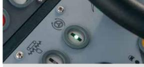
Extreme manœuvrability thanks to Pivot Steer: The rear inside wheel is automatically slowed down hydraulically when Pivot Steer is activated. This minimizes the outside turning circle to not more than 3.5 m for positioning manœuvres and paving.
