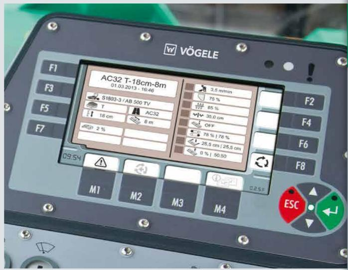
The automatic Paving Programs function allows the operating personnel to store their own paving programs. All the key parameters for paving a specific layer, e.g. a base course of asphaltic concrete 18 cm thick, can thus be stored.
